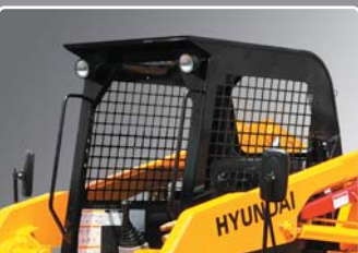
ROPS / FOPS Canopy ROPS : Roll Over Protective Structure FOPS : Falling Object Protective Structure
